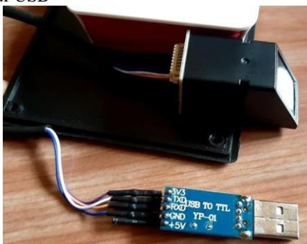
Gambar 12. Fingerprint to Modul USB
