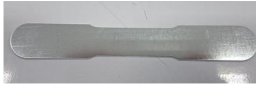
Figure 5. Standard tensile test sample shape. Cut using a punch machine with special dies.
