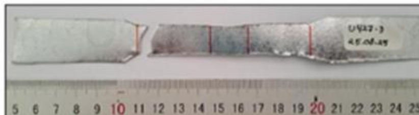
Figure 3. Photo sample with a thickness of 0.45 mm conducted in an independent laboratory
