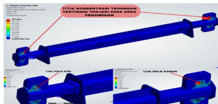
Figure 11. Voltage Distribution of Von Mises Spreader On SM490A Steel.
