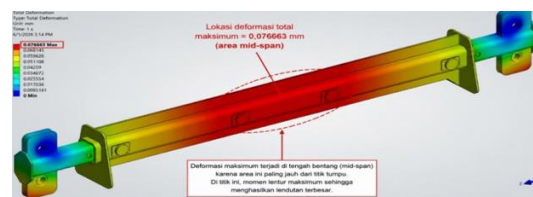
Figure 13. Total Deformation Spreader on SS400 Steel.
