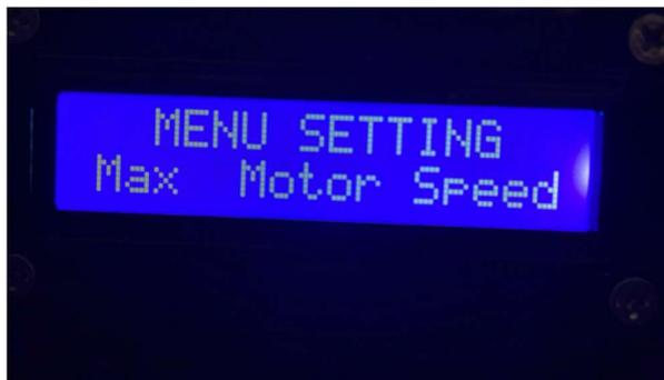
**Gambar 4. 4 LCD 16x2**
