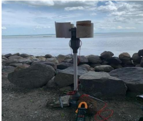
Gambar Pengujian Vertical Axis Wind Turbine
