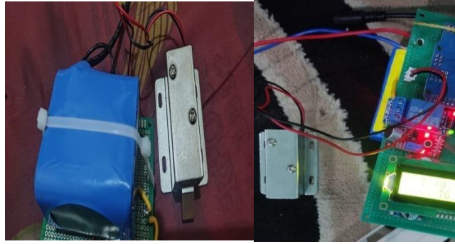
Gambar 4. 4 Pengujian Solenoid Lock.
