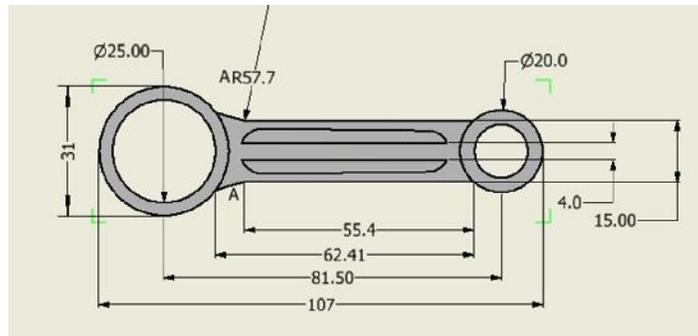
Gambar 3. Ukuran connecting rod
