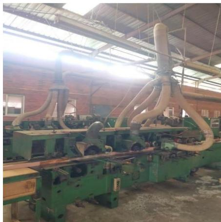
Gambar 7. Mesin *Moulding* Unimat 22 A
