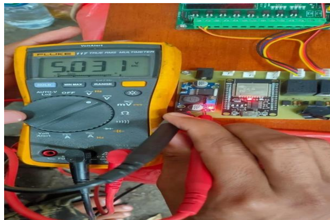
Gambar 3. Pengujian Regulator Step Down
