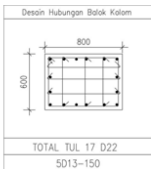
Gambar 16. Desain Tulangan Joint (SRPMK)
