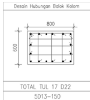
Gambar 16. Desain Tulangan Joint (SRPMK)
