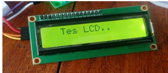
Gambar 4.2 Uji Coba LCD
