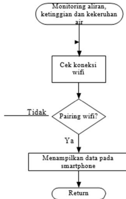
Gambar 4 Flowchart subprogram monitor Blynk
